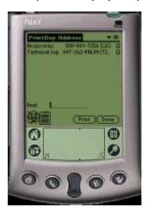
The PrintBoy/Address screen lists all of your Palm addresses by category, just like the built-in Address List application. Use the category dropdown list in the upper right corner of the screen, along with the vertical scrolling feature, to locate the address you wish to print. As an alternative, you can use the Find feature to jump to the address by entering the first few letters in Graffiti.
