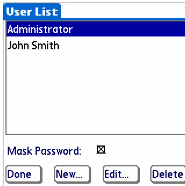
To create a new user, tap on the “New...” button and enter the username and password for the user. If “Mask Password” is selected, the password is not displayed on the screen. You can also leave the password field empty and you will be prompted to enter the password when the Windows logon screen is displayed.
