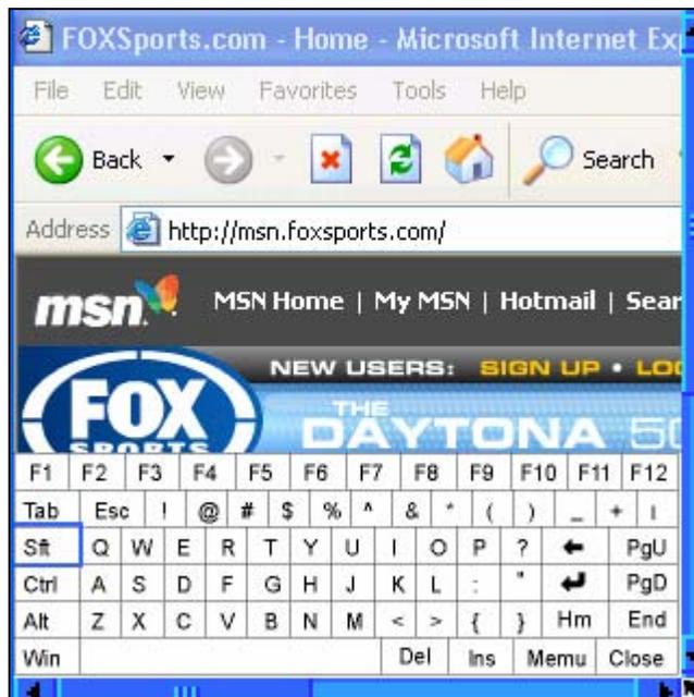
RemotePlus provides a Windows style software keyboard to help you enter special Windows keys and key combinations. You can tap on the arrow at the bottom right corner of the screen or press the MemoPad button to show or hide the software keyboard. Some of the special keys like “Sft”, “Ctrl”, and “Alt” can be toggled to let you enter key combinations using the stylus.
